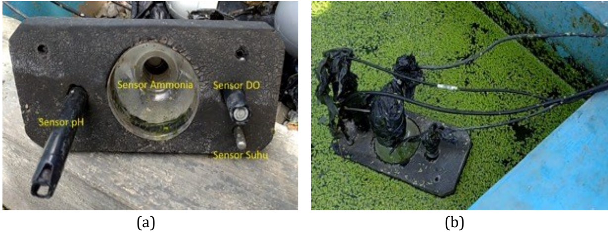
Fig. 11. Water quality sensing module and test setup: (a) sensors used in the system and (b) sensor placement during pond testing.
