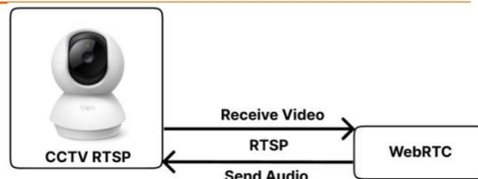
**Figure 6.** CCTV integration using the real-time streaming protocol (RTSP)
