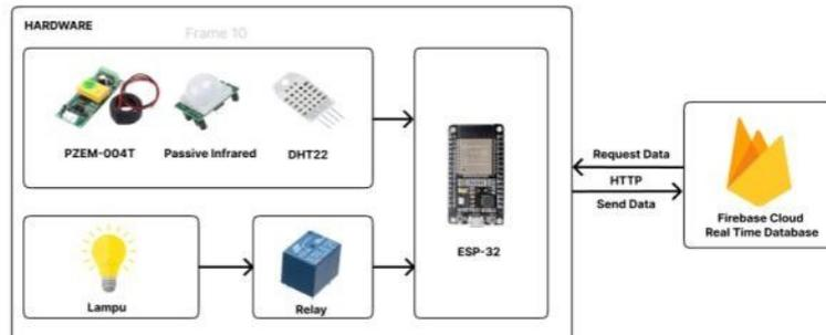
**Figure 4.** Hardware circuit system design
