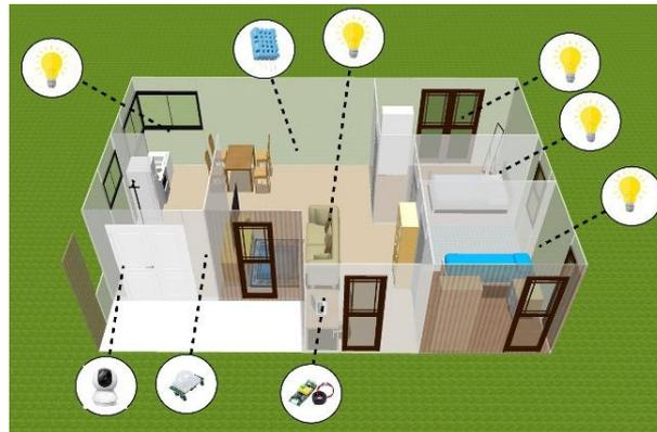
**Figure 2.** Sensor location design
