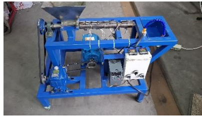
Figure 2. Single Screw Plastic Extruder Machine (used for this research)
