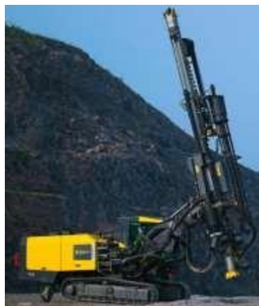
Figure 2. PowerROC T50 COP 3060 Drilling Tool
