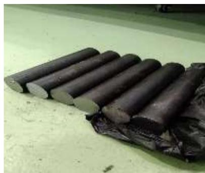
Gambar 4. Spesimen pin track link
