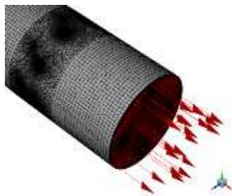
Figure. 8 Results of Hexahedral and Tetrahedral Meshing
