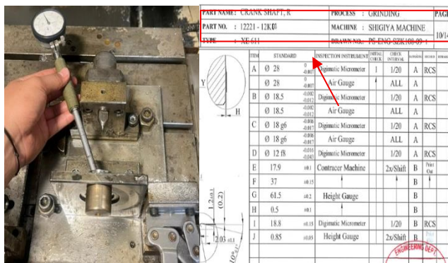
Figure 6. Inspection of Jig Bushing Condition
