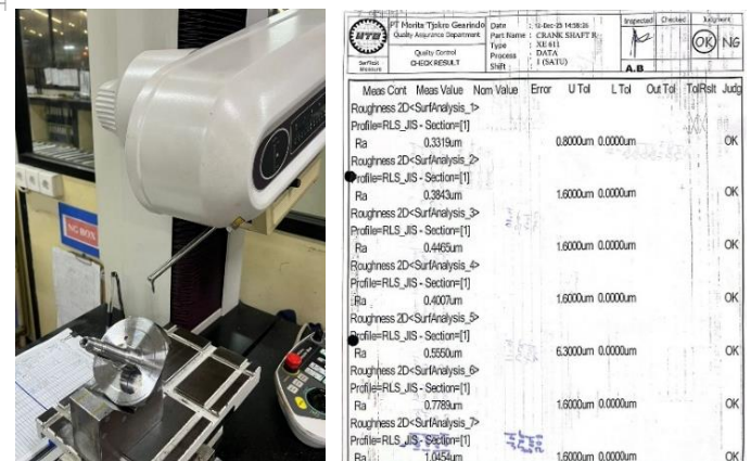
Figure 8. Roughness Inspection Results
