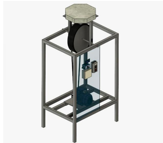
Gambar 2. 3D simulator pendeteksi kerusakan bearing
