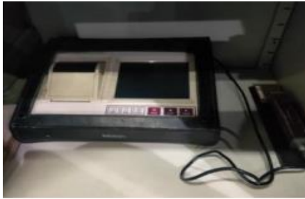
Gambar 2. Mesin Surface Roughness Tester Mitutoyo SJ-310
