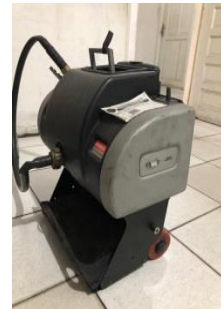
Gambar 2. Gas Analyzer Texa Gasbox Autopower
